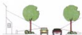
open landscaping allowing natural surveillance from passing traffic
