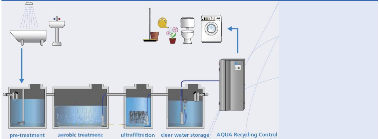
FIGURE C-2: A TYPICAL DOMESTIC GREYWATER RECYCLING SYSTEM
