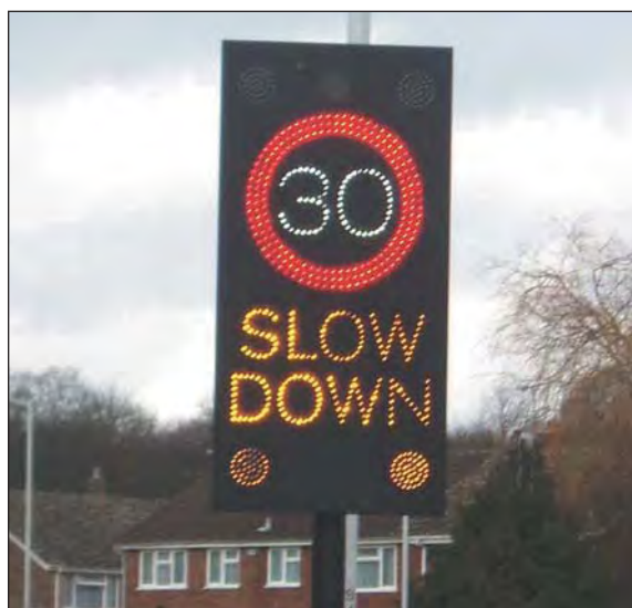
Use of a Vehicle Actuated Sign has reduced speeds by 5 mph at this site in Wigmore Lane, Luton.
