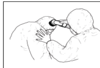
'Buddy' cleaning using a Class H vacuum cleaner
