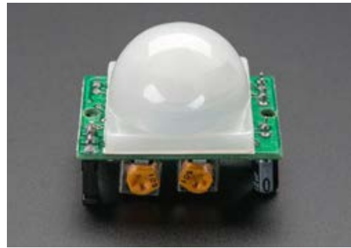
Fig. 1.9.1 Passive Infrared Sensors detect body heat from humans and activate lights when they enter a room.
